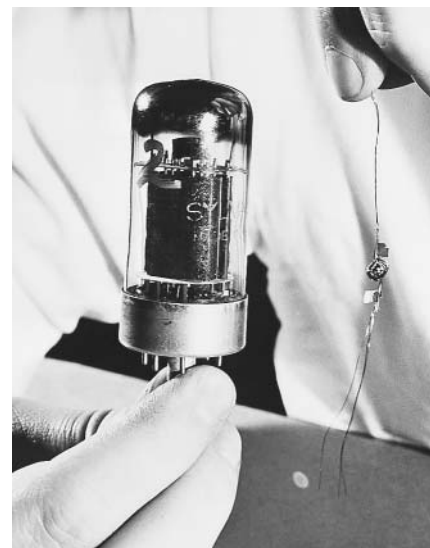
A conventional tube amplifier, at left, and a solid-state memory cell, at right. The size of such semiconductors allows for the manufacturing of smaller devices.
